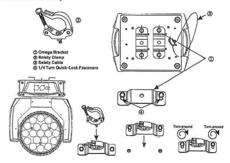
Regardless of the rigging option you choose for your 200W LED spot, always be sure to secure your fixture with a safety cable. The fixture provides a built-in rigging point for a safety cable on the hanging bracket as illustrated above. Be sure to only use the designated rigging point for the safety cable and never secure a safety cable to a carrying handle.
