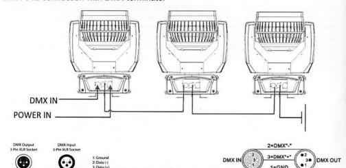
For installations where the DMX cable has to run a long distance or is in an electrically noisy environment, such as in a discotheque, it is recommended to use a DMX terminator. This helps in preventing corruption of the digital control signal by electrical noise. The DMX terminator is simply an XLR plug with a 120  $\Omega$  resistor connected between pins 2 and 3,which is then plugged into the output XLR socket of the last fixture in the chain. Please see illustrations below.
